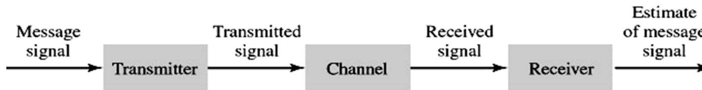
Figure 1.2: Elements of a communication system. The transmitter changes the message signal into a form suitable for transmission over the channel. The receiver processes the channel output (i.e., the received signal) to produce an estimate of the message signal.
