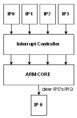
IP0, IP1, IP2, and IP3 raised interrupt request (IRQ) at the same time. The IRQs are sent to the interrupt controller.
