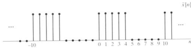
Figure 8.1 Periodic sequence with period N = 10 for which the Fourier series representation is to be computed.
