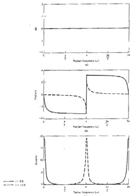
Figure 5.19 Frequency response for allpass filters with real poles at z = 0.9 (solid line) and z = -0.9 (dashed line). (a) Log magnitude. (b) Phase (principal value). (c) Group delay.
